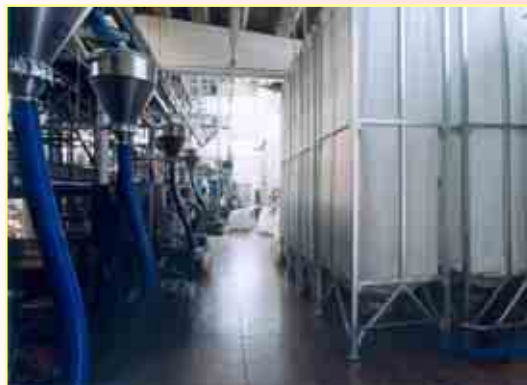
Installation with product dosing from more stations
