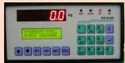
Electronics for the management of 12 silos and planning of 50 recipes
